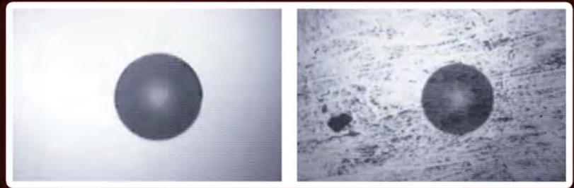
Above: Clean connector face (left), Dirty connector face (right)
